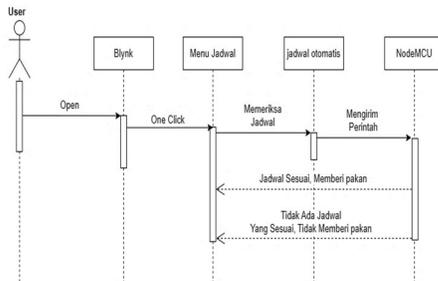
Gambar 6 Sequence Diagram Otomatis
