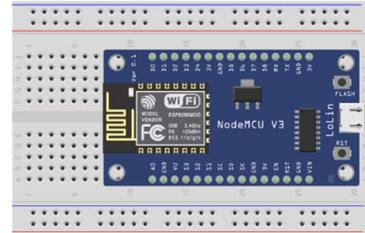
Gambar 8 NodeMCU ESP8266 ke Breadboard
